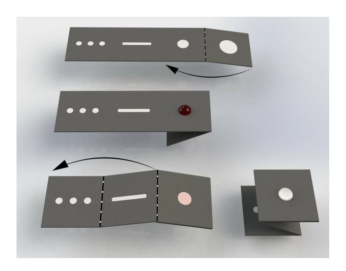
Paper-folding steps for fluidic manipulation. Schematics of how the paper strip in the microfluidic device is folded for each step. The arrows indicate the direction of folding. Credit: Niall P. Macdonald (Dublin City University, Dublin)
