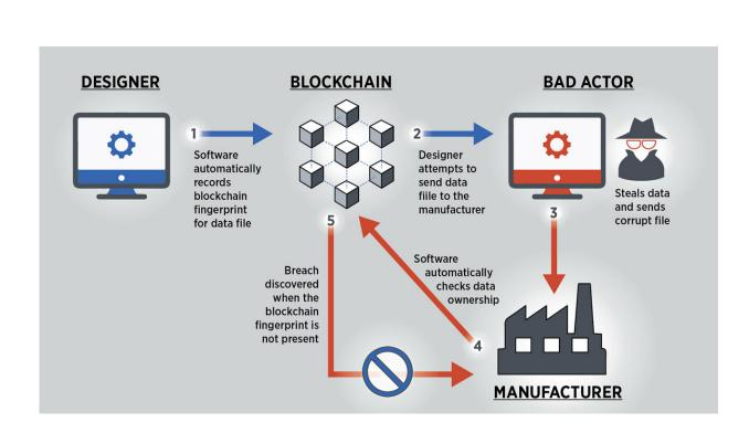
Blockchain technology could help deter digital threats in smart manufacturing systems. Credit: N. Hanacek/NIST
