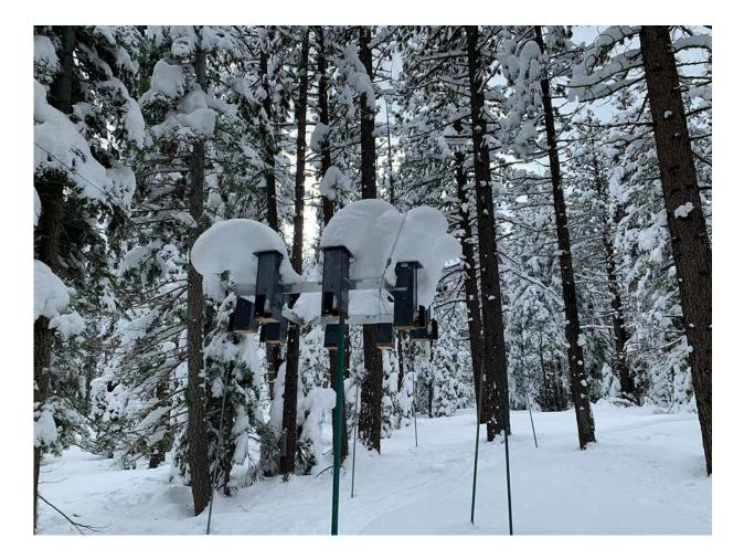
The field lab at high elevation is the centerpiece for this study, with two identical metal frameworks - arrays - that hold eight feeders each. Access to the feeders is regulated by RFID activated doors and the feeder arrays can be raised and lowered depending on the snow depth. Credit: Vladimir Pravosudov, University of Nevada, Ren.
