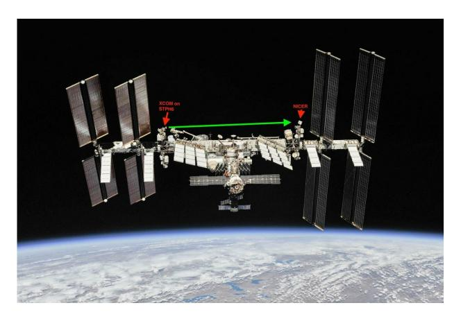
NASA's first-ever demonstration of X-ray communication will occur on the International Space Station. This image shows the locations of the Modulated X-ray Source and the Neutron star Interior Composition Explorer, or NICER, which are critical to the demonstration. Credit: NASA
