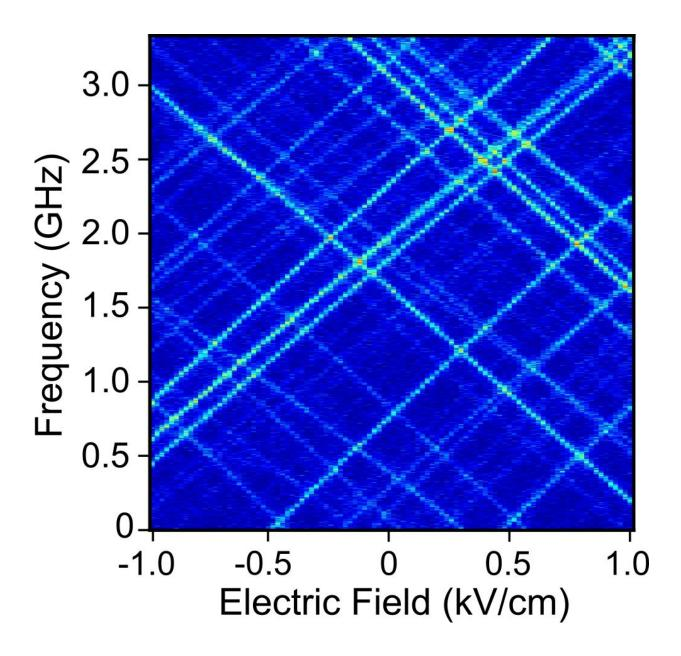
Figure 2. The spectral lines are strongly affected by an electric field. (In the absence of an electric field they are horizontal, see fig. 1.) The frequency change gives away the presence of an electric field. One electron generates an electric field that is 1.5 kV/cm at 100 nm distance, so the frequency shift would be large enough to detect this field.
