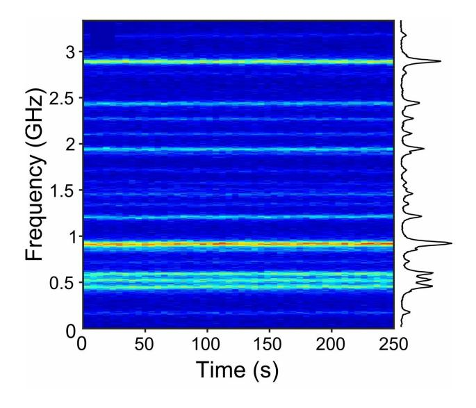
Figure 1. Fluorescent spectral lines of multiple DBT molecules in the absence of an electric field. The lines keep a stable frequency over time.
