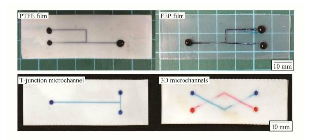
Representative fluoropolymer microchannels that are filled with water containing aqueous dyes. Credit: SUTD
