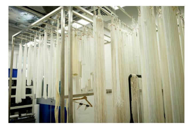
START Centre is a a national-level facility in Singapore to develop and commercialise innovative separation and filtration technologies. This is a membrane production line at START Centre, which produces the tri-bore hollowfibre membrane being commercialised by START Centre and Memsift Innovations.
