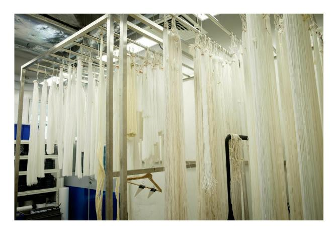
START Centre is a a national-level facility in Singapore to develop and commercialise innovative separation and filtration technologies. This is a membrane production line at START Centre, which produces the tri-bore hollow-fibre membrane being commercialised by START Centre and Memsift Innovations.
