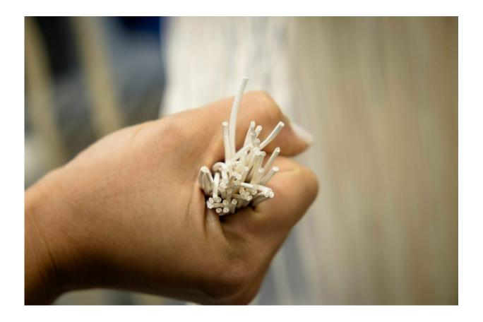
Close up shot of the tri-bore hollow-fibre membrane commercialised jointly by START Centre and Memsift Innovations, which will be used in a new pilot wastewater treatment plant for a semiconductor factory in Singapore. Credit: Nanyang Technological University
