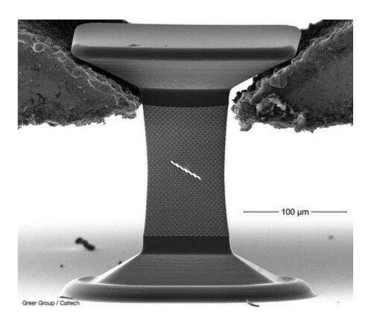
An architected material is strength-tested by stretching until failure. Credit: Greer Group / Caltech
