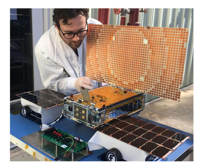
Engineer Joel Steinkraus uses sunlight to test the solar arrays on one of the Mars Cube One (MarCO) spacecraft at NASA's Jet Propulsion Laboratory. Credit: NASA/JPL-Caltech
