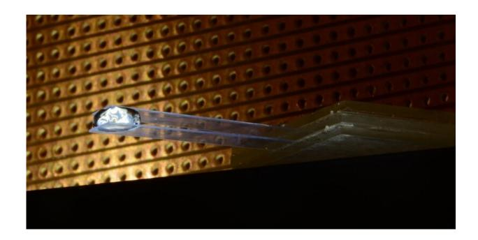
Self-driving drops. Researchers demonstrate that liquid drops will move themselves along a narrow, flexible channel created by two glass coverslips that are clamped at one end. The mechanism may be useful in lab-on-a-chip technologies. Credit: F. Box/Univ. of Oxford
