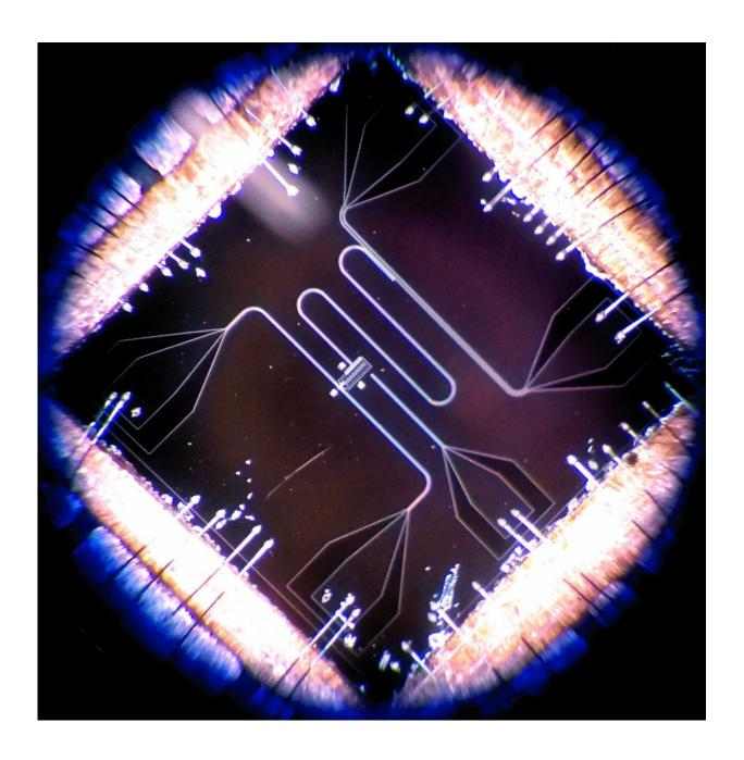
Superconducting circuits comprising a transmon device can be used for quantum
