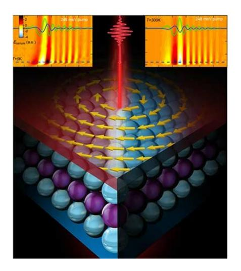
By employing ultra-short mid-infrared and terahertz pulses of less than one trillionth of a second, researchers at Ames Laboratory were able to successfully isolate and control the surface properties of a bismuth-selenium (Bi<sub>2</sub>Se<sub>3</sub>) 3-D topological insulator. Credit: Ames Laboratory
