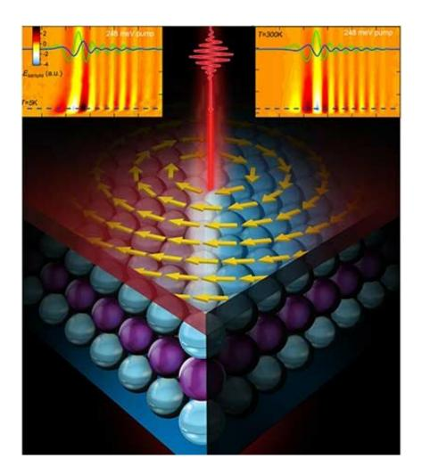
By employing ultra-short mid-infrared and terahertz pulses of less than one trillionth of a second, researchers at Ames Laboratory were able to successfully isolate and control the surface properties of a bismuth-selenium ( $Bi_2Se_3$ ) 3-D topological insulator. Credit: Ames Laboratory
