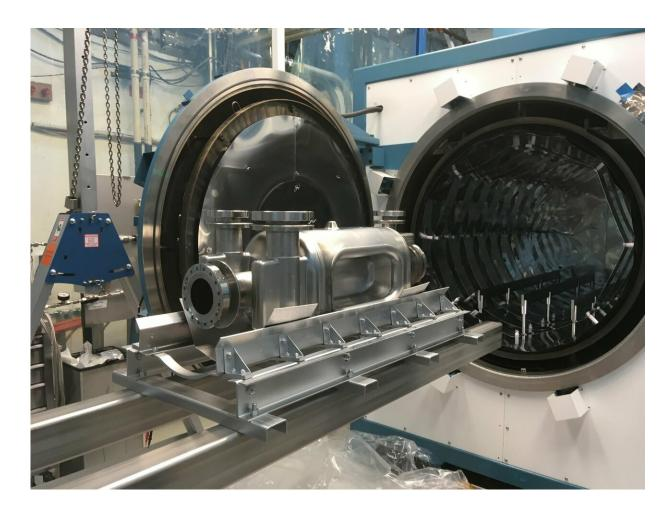
This accelerating cavity is a type known as "crab cavity." It is designed to maximize the chance of collision between two opposing particle beams. Credit: Paolo Berrutti
