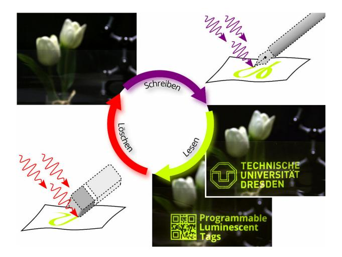
The multiple writing, reading and erasing cycles. The UV-illuminated patterns can be erased by infrared light again and again. Credit: M. Gmelch and H. Thomas, TU Dresden
