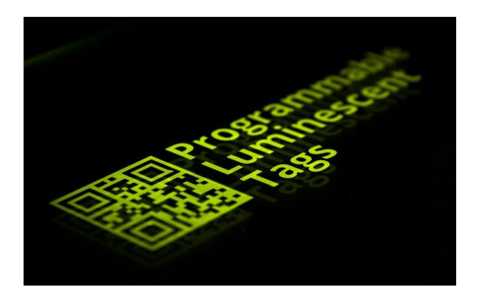
A luminescent tag, contactless printed onto a plastic foil. The light emitting layer is thinner than a human hair. The imprint can be erased and replaced by another pattern. Credit: M. Gmelch and H. Thomas, TU Dresden
