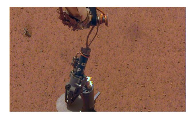
NASA's InSight lander set its heat probe, called the Heat and Physical Properties Package (HP3), on the Martian surface on Feb. 12. Credit: NASA/JPL-Caltech/DLR
