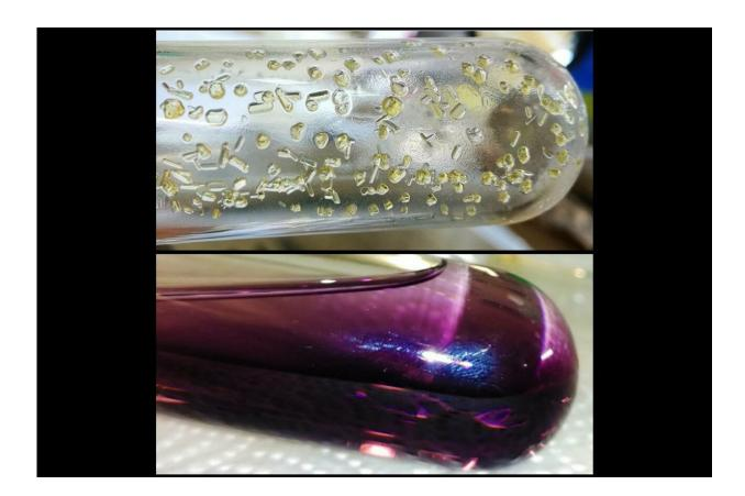
Metal carbonyl complex filled in a bottle. Credit: AG Krossing/J. Bohnenberger
