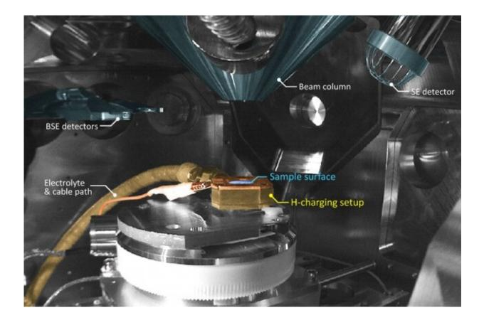
The experimental scanning electron microscope setup used by the researchers to study the hydrogen-loading process. Credit: Massachusetts Institute of Technology
