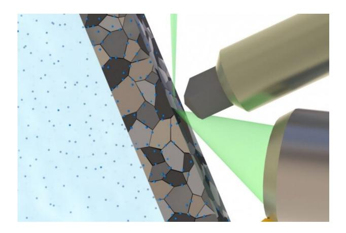
This illustration depicts the main elements of the system the team used: The multicolored slab at center is the metal layer being studied, the pale blue region at left is the electrolyte solution used as a source of hydrogen, the small blue dots are the hydrogen atoms, and the green laser beams at right are probing the process. The large cylinder at right is a probe used to indent the metal to test its mechanical properties. Credit: Massachusetts Institute of Technology
