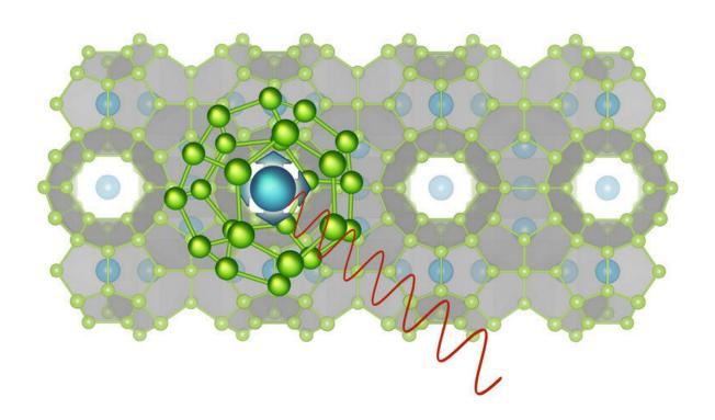
The atom in the cage can oscillate in two different directions. Credit: Vienna University of Technology
