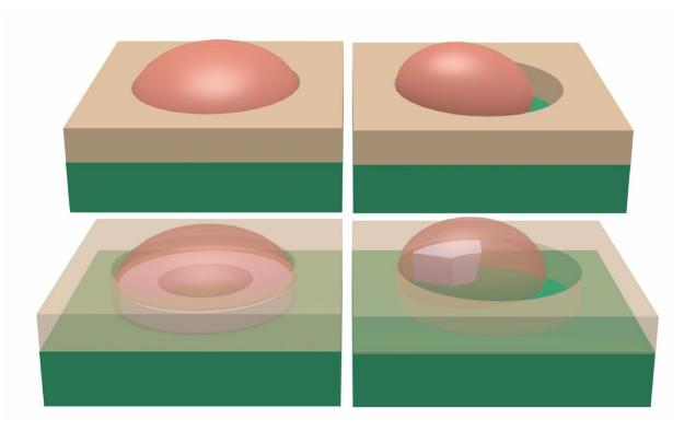
Two different configurations of the droplet within the opening – hole fully filled and partially filled and bellow illustration of GaAs crystals forming a full ring or a step underneath the large and small gallium droplets. Credit: Ecole Polytechnique Federale de Lausanne (EPFL)
