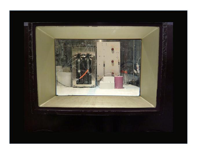
Prototype fluidic system for zirconium-89 purification. Image taken through a hot cell window at the Department of Radiology, University of Washington. Credit: Matthew O'Hara, Pacific Northwest National Laboratory
