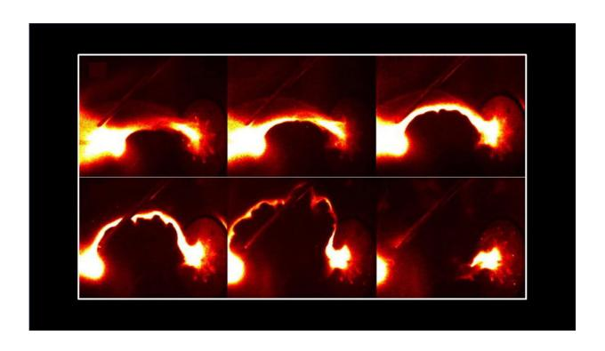
Rapidly accelerating kink instability (arch shape) of a plasma jet produces an effective gravity that causes "ripples" (seen on bottom of the arch). The ripples choke the jet at which time a burst of 6 kilovolt X-rays is observed. The whole process lasts a few microseconds, and the X-ray burst is approximately one microsecond in duration. Credit: Ryan Marshall and Paul Bellan
