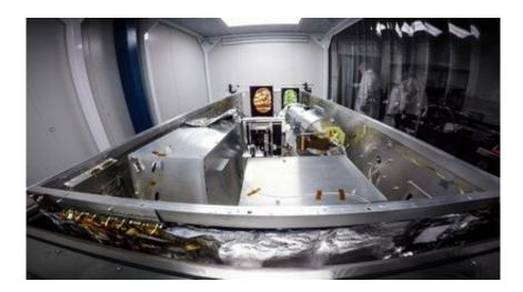
The new Penn State-led Habitable Zone Planet Finder (HPF) provides the highest precision measurements to date of infrared signals from nearby stars. Pictured: The HPF instrument during installation in its clean-room enclosure in the Hobby Eberly Telescope at McDonald Observatory. Photo Credit: Guðmundur Stefánssonn, Penn State
