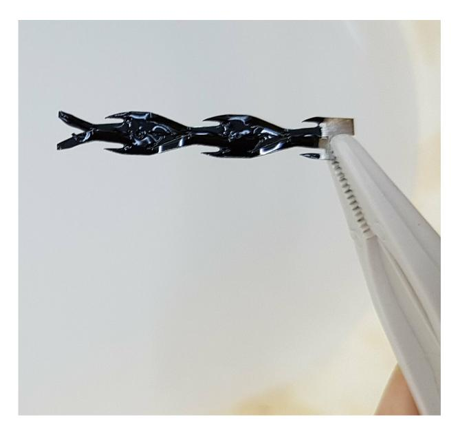
GraphON coated catalytic static mixer. Credit: CSIRO
