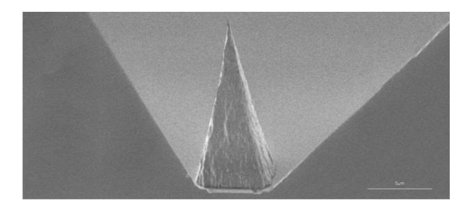
An example of one of the diamond pyramid tips used in the experiments. The tip has a radius of 10 nanometers allowing sensing with nanoscale spatial resolution. Credit: Adapted with permission from Ref 1. Copyright (2018) American Chemical Society
