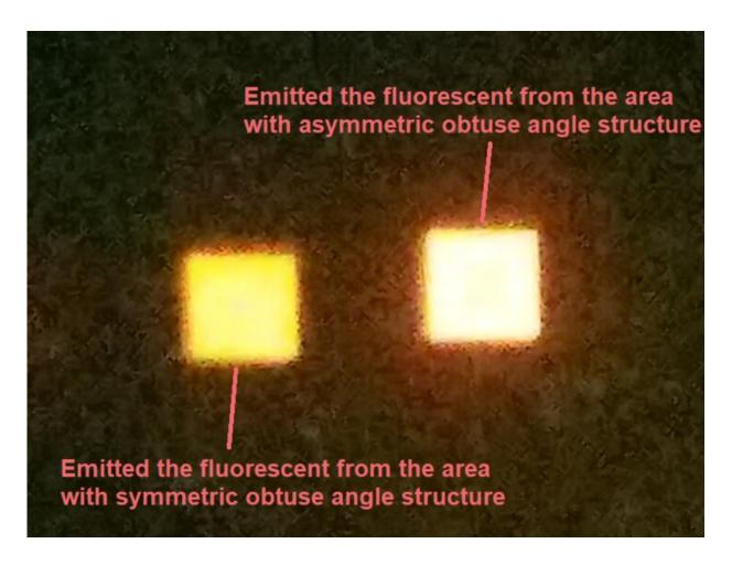
Comparing the light that was emitted from symmetric and asymmetric structures. Credit: Pennsylvania State University
