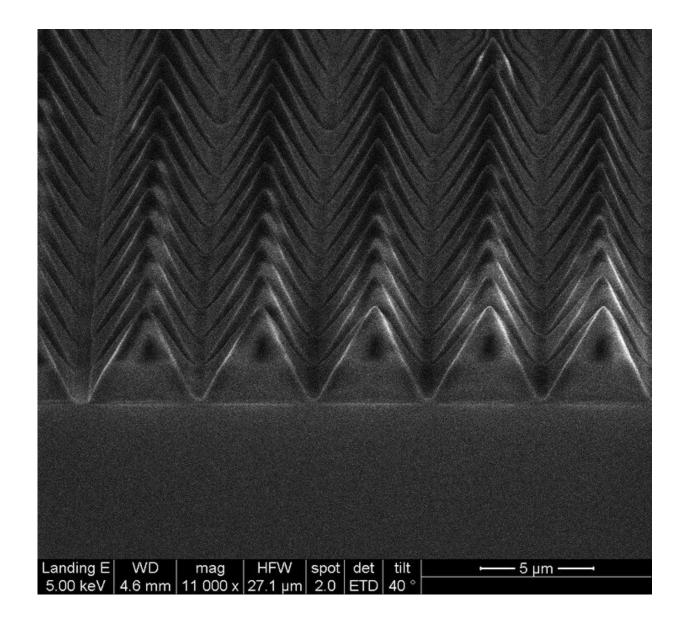
Scanning electron microscope image of the symmetric pyramids that were 3-D naonprinted. Credit: Pennsylvania State University
