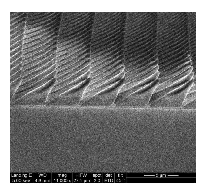
Scanning electron microscope image of the asymmetric pyramids that were 3-D naonprinted. Credit: Pennsylvania State University
