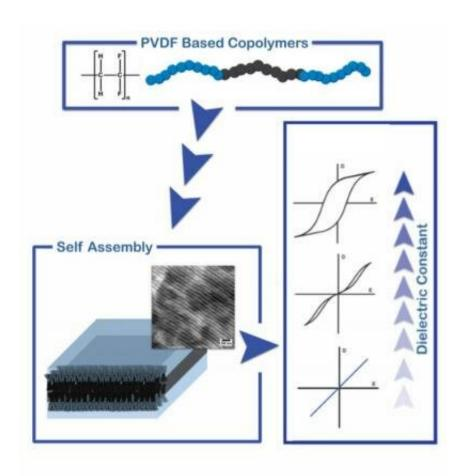
A block copolymer of PVDF (black) and an insulating polymer chain (blue) form a block copolymer. Through phase separation, the blocks assemble in films. The dielectric properties can be tuned by varying composition and length of the blocks. Credit: Department of Polymer Science, University of Groningen
