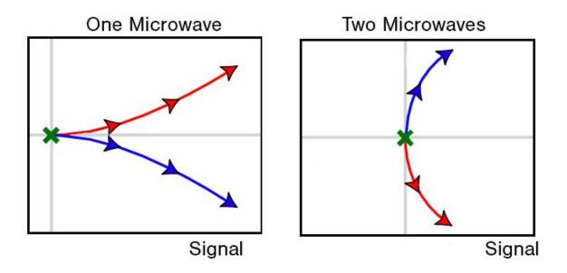
The speed at which the two states of the qubit separates is much faster when probed with two microwaves Credit: Aalto University
