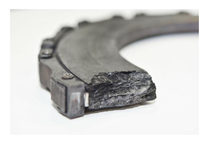
Aircraft brake disk, breakage after machanical tests Credit: Sergey Gnuskov/NUST MISIS
