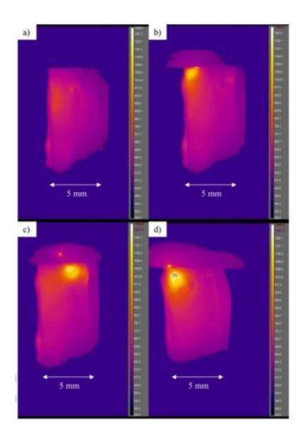
Another surprising observation of electric heating of glass is that the hot spot near the positive electrode may meander around as seen in the video frames several seconds apart in the figure here. Credit: Himanshu Jain, Nicholas J.
