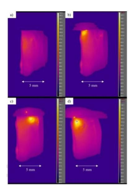
Another surprising observation of electric heating of glass is that the hot spot near the positive electrode may meander around as seen in the video frames several seconds apart in the figure here. Credit: Himanshu Jain, Nicholas J.
