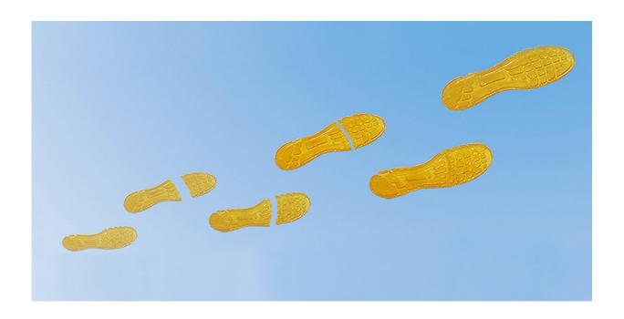
Severed 3D-printed shoe pad repairing itself. Credit: An Xin and Kunhao Yu
