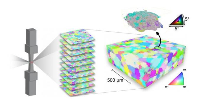
The evolution of the internal microstructure of a nickel-titanium sample is measured while it is mechanically tested. The colors correspond to crystallographic orientation, and the orientations are clustered into grains, or crystals. Credit: Colorado School of Mines
