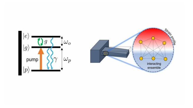
(left) Model of cooling cycle: an external laser pumps atoms into a two-level subspace coupled directly to a mechanical resonator; phonon absorption results in cooling of the mechanical system. (right) Schematic of a mechanical resonator interacting with an atomic ensemble. The engineered strain profile couples to dark entangled states of the ensemble resulting in optimal cooling. Credit: Argonne National Laboratory
