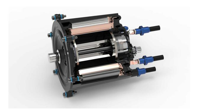
Sectional view of the electric motor. The core of the motor is a stator consisting of twelve individual teeth, which are wound upright using a flat wire. Credit: Fraunhofer ICT
