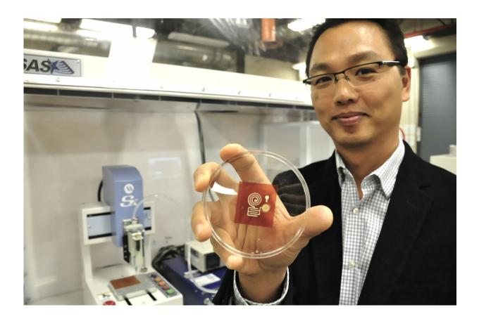
SFU Mechatronic Systems Engineering professor Woo Soo Kim is collaborating with Swiss researchers to develop an eco-friendly 3D printable solution for producing wireless Internet-of-Things sensors. The research team is using a wood-derived cellulose material to replace the plastics and polymeric materials currently used in electronics. Credit: SFU
