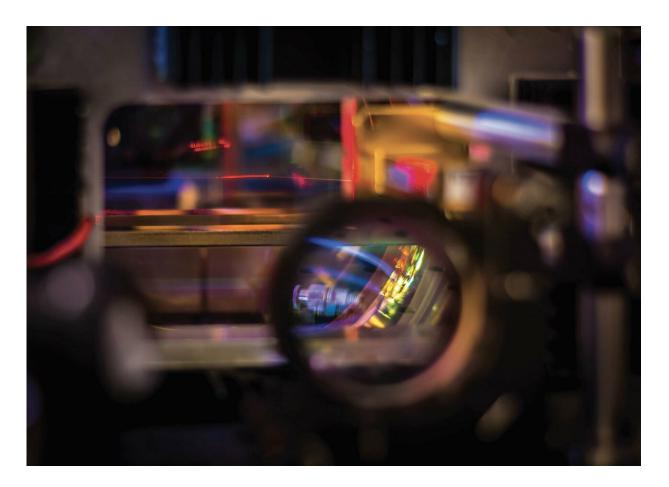
Picture of an optical nanofiber (in red) inside a vacuum chamber. Arrays of individual cold atoms can be trapped around the fiber -about 200 nanometers from the surface- and addressed via the guided light. These "fibered atoms" offer an integrated platform for quantum information networks and for waveguide-QED investigations. Credit: Kastler Brossel Laboratory– N.V. Corzo.
