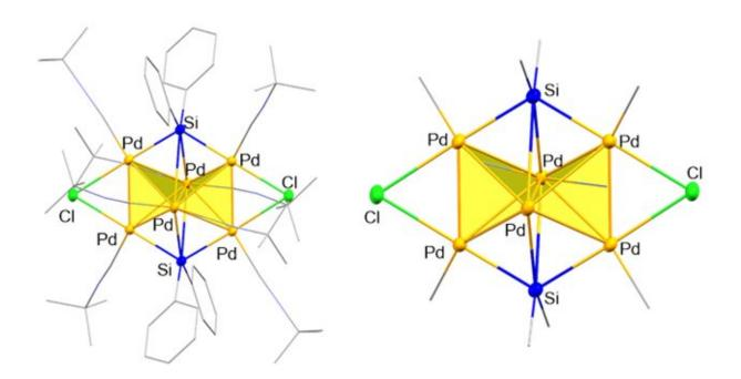
The entire (left) and the core (right) structure of 3-D cluster molecule based on palladium. Credit: 2019 Yusuke Sunada, Institute of Industrial Science, The University of Tokyo
