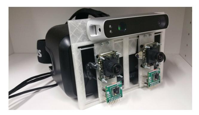
Scientists have developed a prototype infrared camera that is triggered when the wearer squints their eyes. Image Credit - Amplify project
