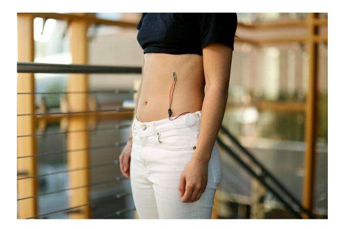
The paired sensors -- one placed between the ninth and 10th ribs and the other on the abdomen -- track the rate and volume of the wearer's respiration by measuring the local strain on the application areas. Credit: Josh Kim / UCI
