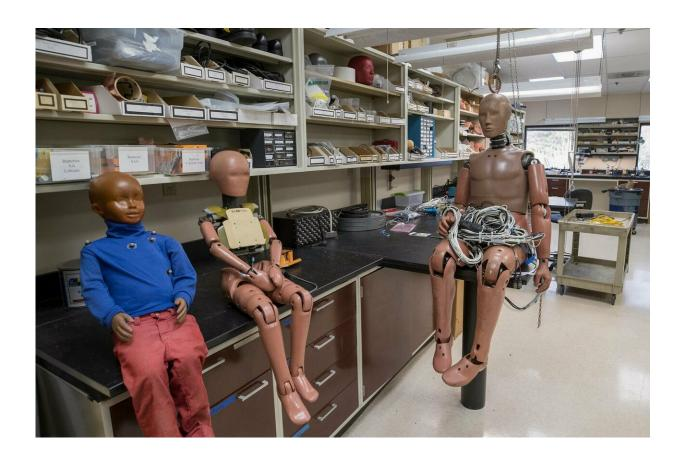
The Center for Applied Biomechanics works with a variety of crash test models to improve automobile safety. Credit: Dan Addison, University Communications
