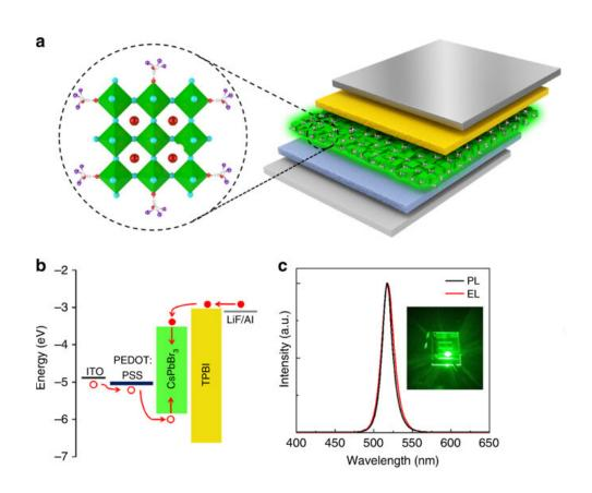
a) Device structure and a corresponding cross-sectional TEM image of the multi-layer PeLEDs; b) Schematic flat-band energy diagram of the PeLED; c) Normalized photoluminescence spectrum of the CsPbBr3 film, and electroluminescence spectrum of the PeLED at an applied voltage of 5.5 V Credit: City University of Hong Kong
