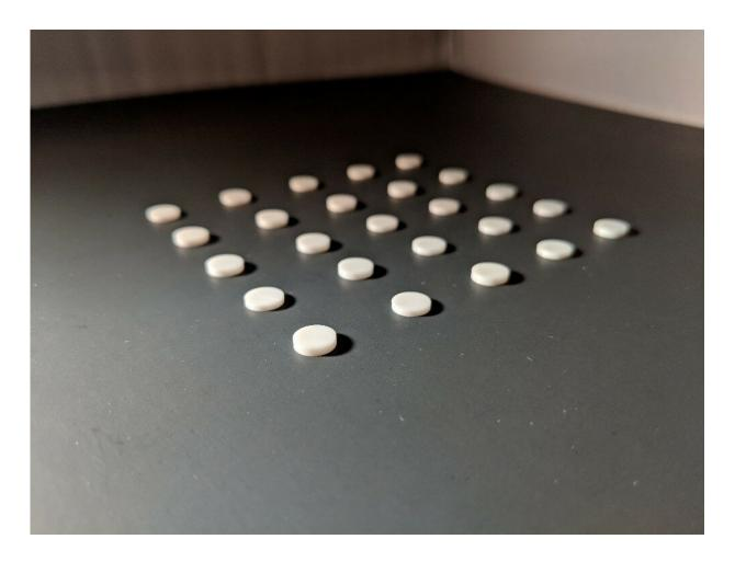
Picture of the actual metamaterial consisting of a field of specifically tailored cylinders. Credit: Willie Padilla, Duke University
