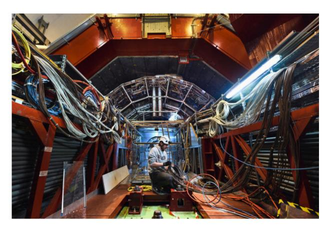
Work has begun on the inner sub-detectors of the ALICE experiment ahead of the installation of new equipment. Credit: Maximilien Brice/Julien Marius Ordan/CERN
