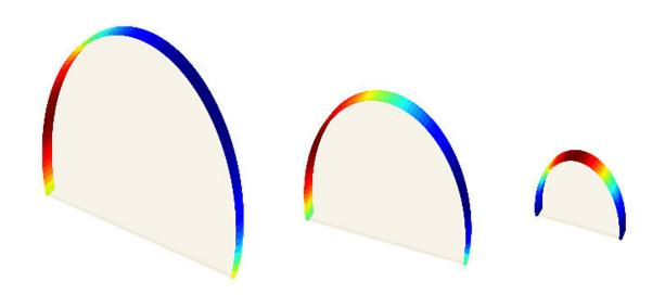
This image illustrates the actual predictions of geometric shape deviations for 3-D vertical semi-cylinders that are generated from Purdue University machine learning technology. Credit: Purdue University
