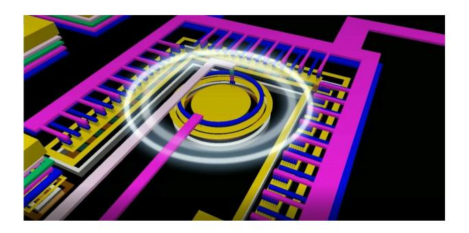
Artist impression of the optocoupler, the round structure is the detector (Single Photon Avalanche Diode), the light source (Avalanche Mode LED) has the shape of a horse shoe. Credit: University of Twente
