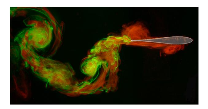
The best wing shapes, such as the one shown above, are found to make strong vortices at the trailing edge that were not interfered with by the vortices generated at the leading edge. Pictured is from an experiment revealing ideal airfoil shapes for flapping flight, with the flows generated at the front part of the wing [red] and the rear [green] visualized using fluorescent dyes. Credit: The Applied Math Lab, NYU's Courant Institute of Mathematical Sciences
