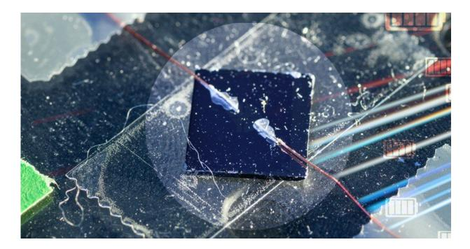
The dark square in the center is a thin film of germanium tin semimetal, with copper wire electrodes, and is undergoing electrical and optical measurements for the possible presence of Weyl fermions. Credit: University of Delaware
