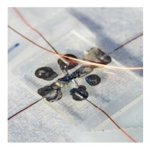
A sample of the Weyl semimetal molybdenum telluride, surrounded by circular contact pads and copper wire electrodes, for an investigation of electrical and optical devices based on Weyl fermions. Credit: University of Delaware
