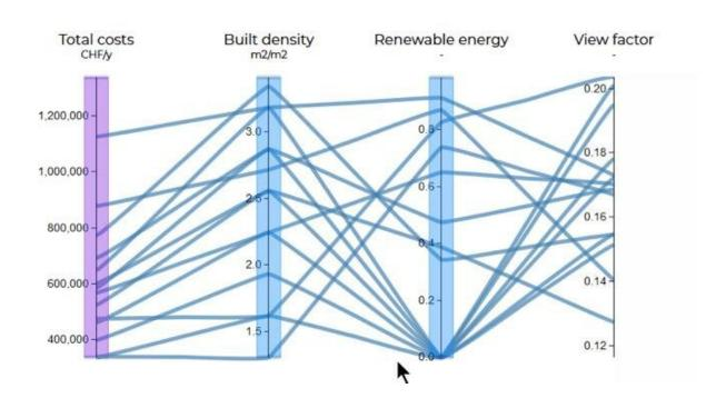
Each horizontal line represents a variant, clearly indicating the variant's score on different criteria such as total cost, built density and use of renewable energy. Credit: Ecole Polytechnique Federale de Lausanne
