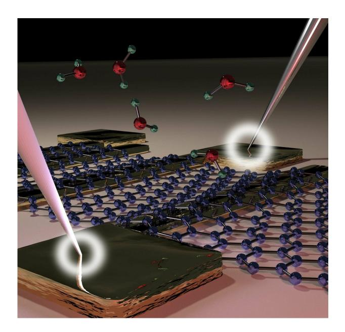
Schematic of a graphene device with a contact resistance that is not altered by the water molecules adsorbed on its surface. Credit: Anderson D. Smith
