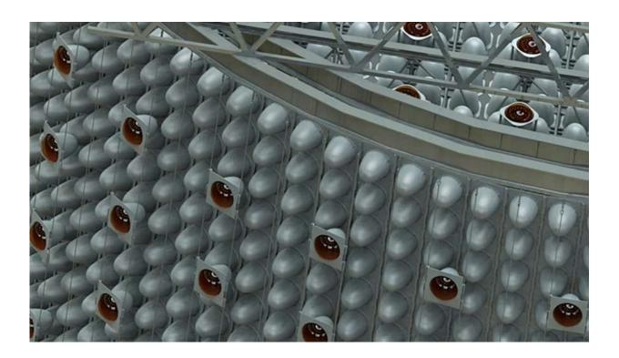
This graphic shows the detail of a possible configuration of the photomultiplier tube mounting structure for the WATCHMAN antineutrino detector, a key part of the Advanced Instrumentation Testbed. Modules containing sets of photomultiplier tubes are securely bolted to cables, which run the vertical length of the detector – like a giant Christmas decoration that absorbs light rather than emitting it. Credit: University of Sheffield
