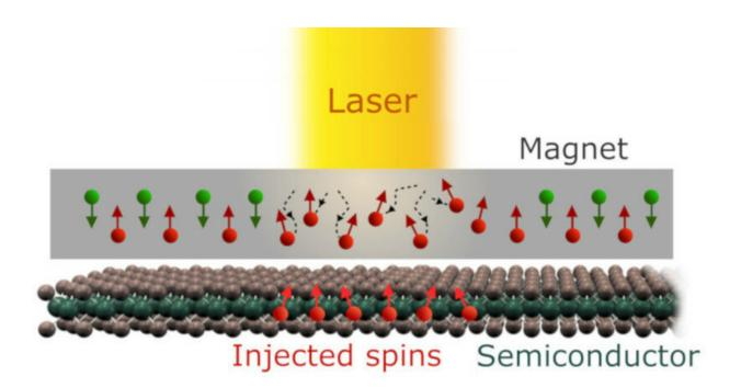
Schematic of the spin-injection experiment. Credit: J. C. W. Song and Y. D. Chong
